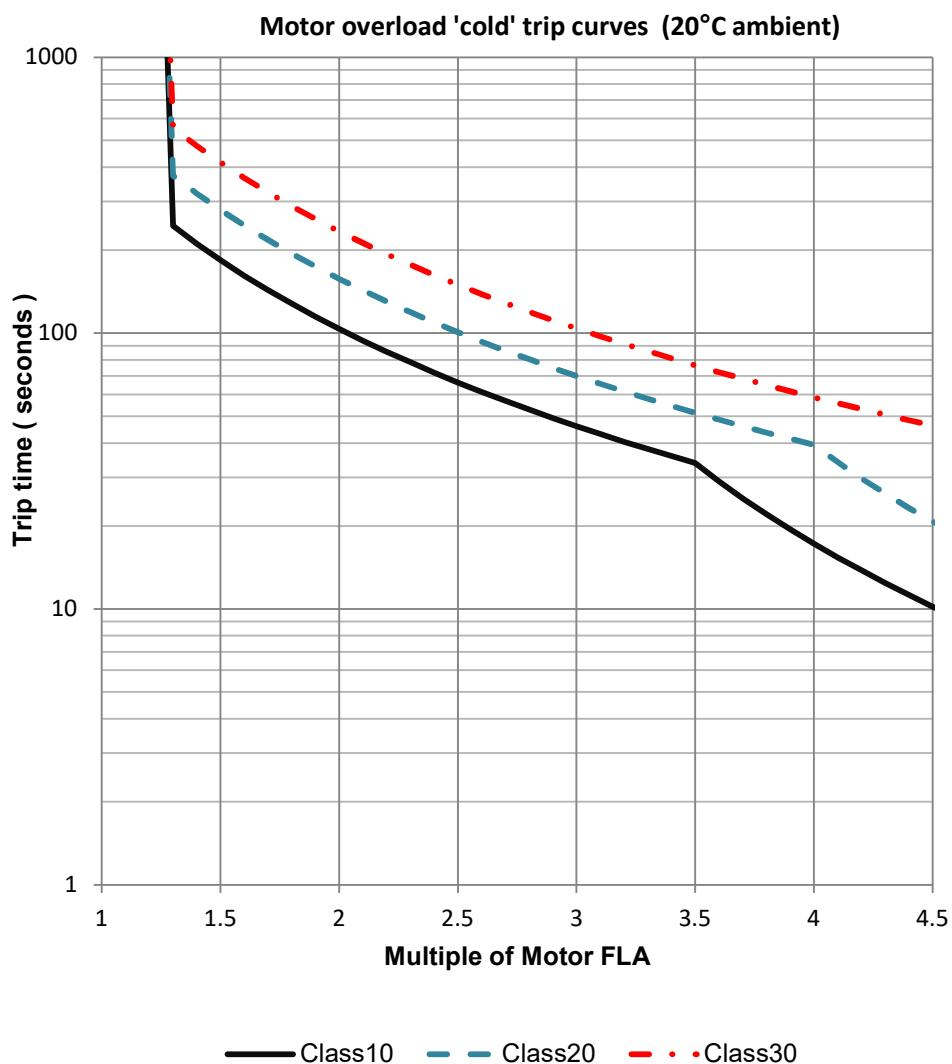
**Note:** When the overload has tripped, there is a forced cooling time to allow the overload to recover before the next start. The 'warm' trip times are 50% of the 'cold' trip time
